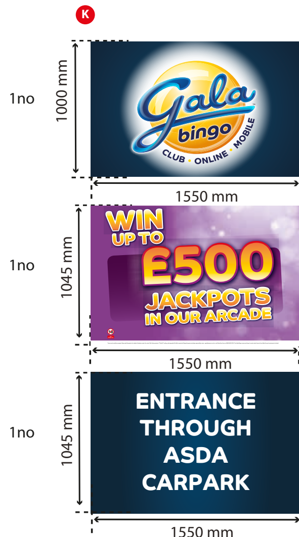
Flat cut aluminium panels powder coated RAL 5011 with print to face. 'entrance through...' to be matt white cut vinyl
